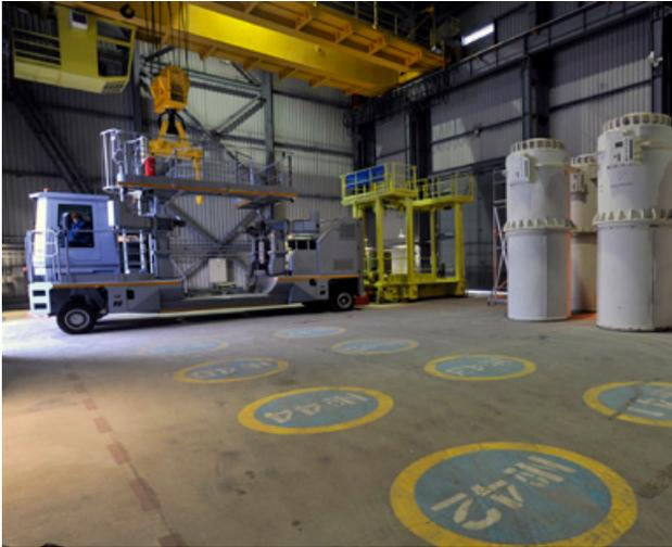
waste. Engineers designed special robotic mechanisms and handling equipment. The robots are used to remove damaged assemblies from the bottom of the spent fuel pool in Building No. 5. Computer simulators were also developed for the operators to train how to hoist out radioactive debris from the blocks and load it into casks and containers. The containers were also developed specially for the project.
