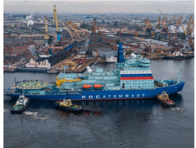
Also on November 22, the Baltic Shipyard in Saint Petersburg put afloat the fourth Project 22220 icebreaker, Yakutia, laid down in May 2020. With RITM-200 reactors and almost all other pieces of core equipment already installed, the ship will be fitted out afloat. Yakutia is planned to be commissioned in December 2024.
