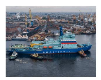
Also on November 22, the Baltic Shipyard in Saint Petersburg put afloat the fourth Project 22220 icebreaker, Yakutia, laid down in May 2020. With RITM-200 reactors and almost all other pieces of core equipment already installed, the ship will be fitted out afloat. Yakutia is planned to be commissioned in December 2024.
