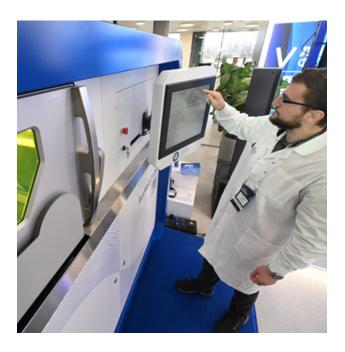
integrating additive manufacturing solutions and services presented Russia's largest 3D printer developed in partnership with the Saint Petersburg State Marine Technical University. Using the direct metal deposition (DMD) technology, the printer can make products weighing up to 6 tonnes, particularly complex-shaped reactor parts. The DMD printer is equipped with two industrial robotic arms and a positioner.
