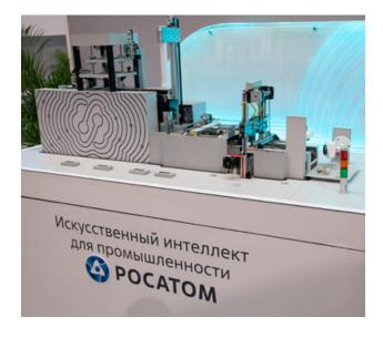
a real production process. The demonstration conveyor was loaded with feedstock (modeling clay), which was analyzed online using various sensors and then processed into a tablet in several stages. The system suggested optimal equipment settings for specific feedstock parameters to reduce scrap and, at the last stage, used video data to determine the quality of the final product.
