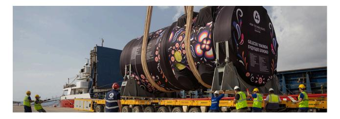
In addition to the reactor pressure vessel, a containment airlock for Unit 3 and a pressurizer for Unit 4 were delivered to the site. The equipment was shipped using various modes of transport. The RPV was delivered to the pier from the manufacturing plant on a self-propelled platform, after which the vessel traveled over 3,000 kilometers by sea to arrive at the Vostochny (Eastern) cargo terminal of the Akkuyu NPP site.
